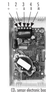
CO 2 sensor electronic board
